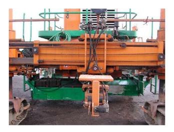
Hydraulic powered float finisher, aluminum/magnesium alloy blade 40cm 16in) wide x 4.00 m (13ft.) long, variable speed for longitudinal finish stroke and lateral travel, hydraulic blade pitch adjustment.
