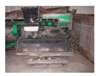
Two paving profile moulds (pan-type) arranged in tandem position, fixed within modular side-form system. Tandem moulds are attached to tractor sub-frame and end-frames permitting mainframe telescopic action to reposition the moulds laterally for adjustment to paving width. Paving width adjustment requires a minimum of labor and tools. Provisions for integral curb mold inserts are provided on both sides.
